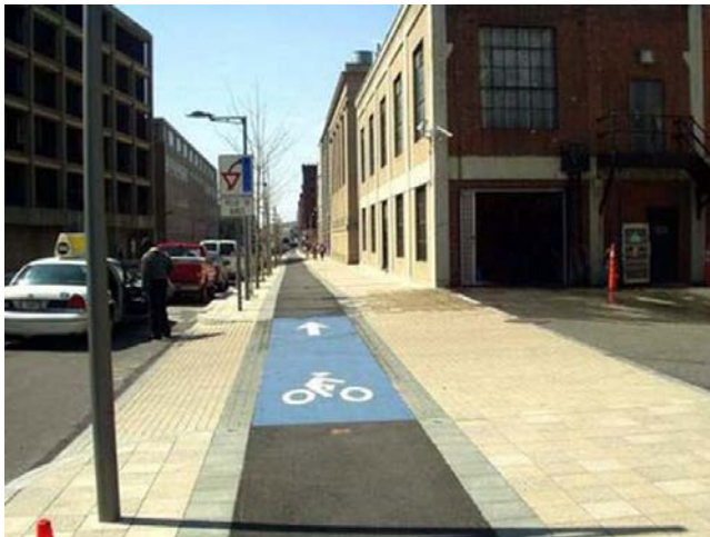
One-way Street Sidewalk Level Cycle Track in Cambridge, MA 12
